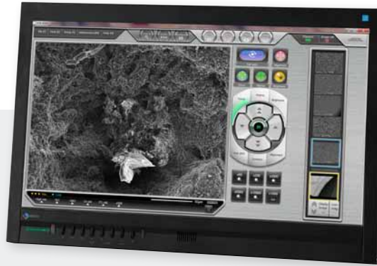
Morgan Advanced Materials take ceramic fault diagnosis to the next level. Picture shows a defect on the surface of an alumina component on the screen of the Nikon Metrology JCM-6000 NeoScope.
